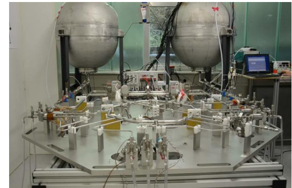
Propulsion feed system hydraulic mock-up used to investigate water-hammer effects, thruster cross-talk etc.
